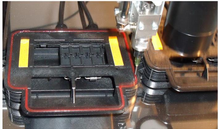
*Applying silicon at the backside of the junction box*
